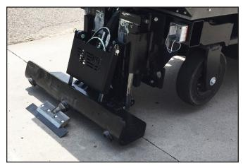
Decreased blade tilt angle and raised blade. Front caster wheels off ground.
