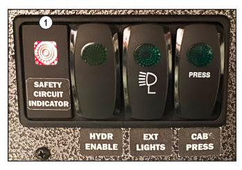
(1) Safety circuit indicator lit up indicating the hydraulic system is disabled.
