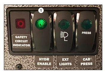
Hydraulic enable switch "ON" indicating the hydraulic system is enabled.
