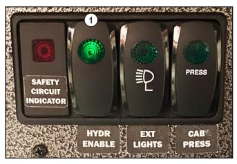
(1) Hydraulic enable switch "ON" indicating the hydraulic system is enabled.
