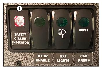
Safety circuit indicator lit up indicating the hydraulic system is disabled.
