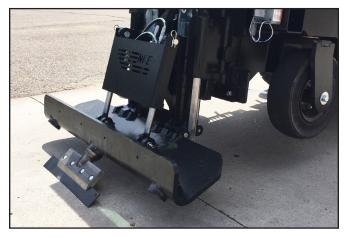
Increased (steep) blade tilt angle and lowered blade. Front caster wheels high off ground.
