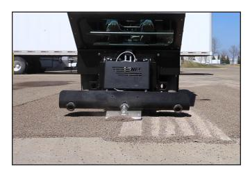
Machine scraping epoxy-covered concrete.
